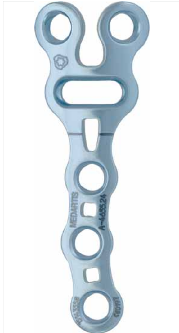
Fig. 24.2 Rotational plate with offset holes to prevent bone splitting and screw collision. Mark for the osteotomy, 1.5-mm plate thickness 0.8 mm for phalangeal correction, and 2 mm with plate thickness 1.3 mm, 1.5 and 2.0 Trilock screws polyaxial with 15 degrees of freedom. (Agreement by Medartis Basel, Switzerland)
